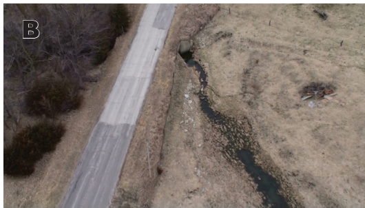
B Medium: No significant bank erosion, but it appears that cattle have disturbed the stream bed.
