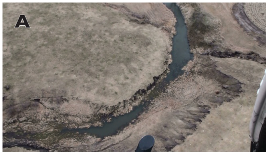
Stage 3. Channel appears to be incising. A nick point is visible in upper right corner of image.
