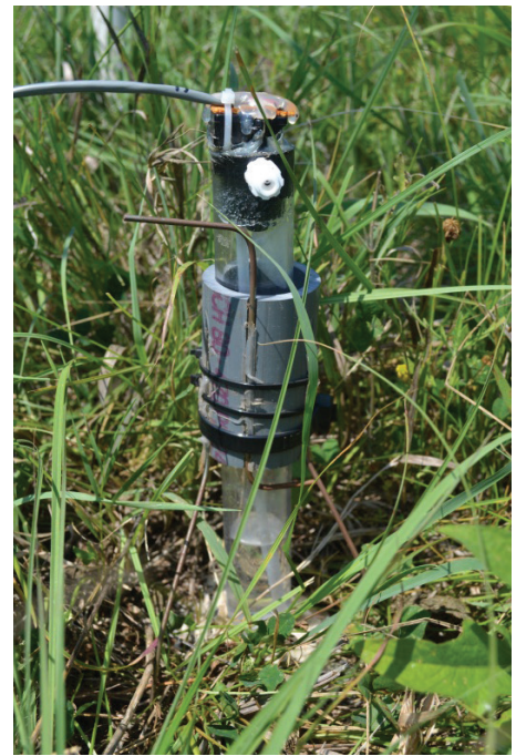
Figure 2. Soil sampling was completed by coring with a hydraulic truck-mounted soil probe, and infiltration measurements were collected using an automated mini disk infiltration network.
